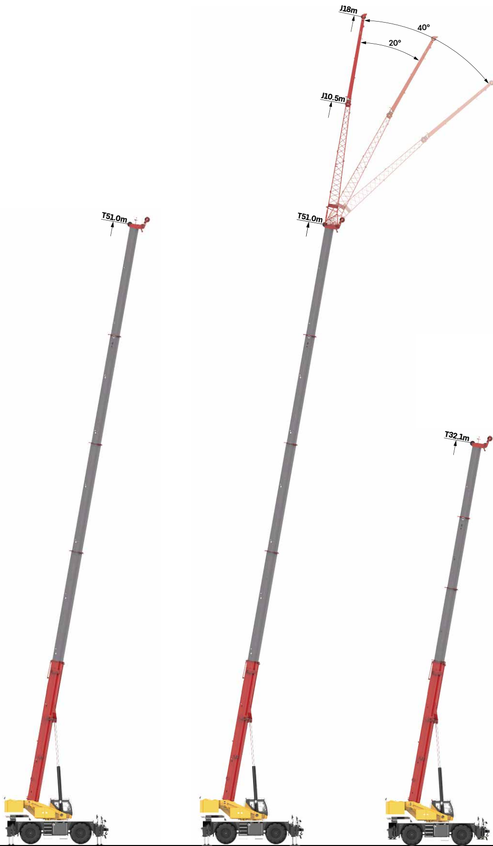
Telescopic boom on outriggers 主臂、支腿吊载
